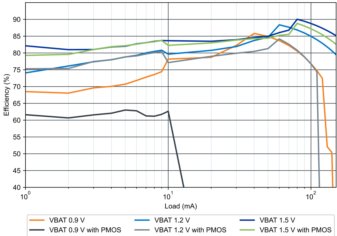
Figure 5: Efficiency comparison of PMOS with 1.5 V battery, 1.8 V VOUT
